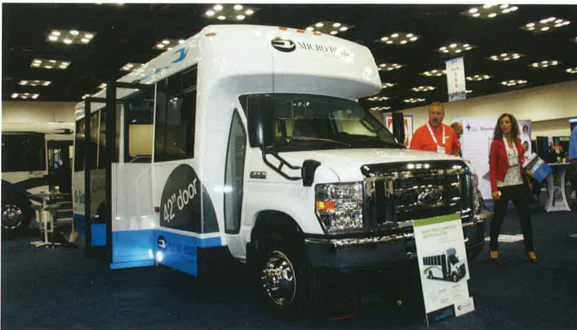
The Micro Bird D-Series MD was one of four buses on display at BusCon by Blue Bird. It featured a wide 42-inch door as well as propane power provided by ROUSH CleanTech. It was built on a Ford E-350 chassis.
